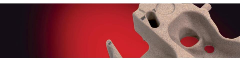
Foseco offers a broad range of organic and inorganic mould and core binder systems. Organic binders are almost exclusively synthetic resins, which are cured by the addition of a separate hardener or catalyst. Inorganic binders are based on sodium silicates that have been optimised to accommodate the varying casting processes, thus guaranteeing best decomposition.
