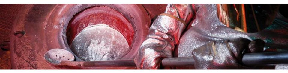
Crucibles are used in a wide range of melting and holding applications for non ferrous alloys, particularly aluminium, copper and zinc. Each of these applications requires a crucible with specific properties to maximise productivity and minimise energy costs.
