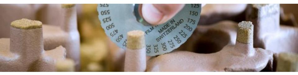
By careful selection of refractory fillers and rheological technology, Foseco coatings are designed to deposit the correct coating structure onto a given substrate, to ensure cast surface integrity. The range of products have been specifically engineered so that they can be applied by dipping, flow coating, brushing, swabbing and spraying.
